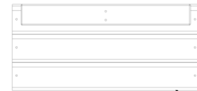
WP7 | CLOISON CENTRALE ARRIÈRE SUPÉRIEURE - W2A03696 (x1) | 1 1/2"x21 1/8"x9 3/4" (38x536x248)
